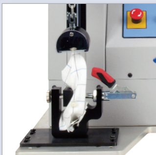
Button pull-off test
