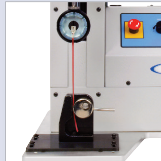
Wire crimp terminal pull-off test
