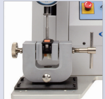
Automotive switch compression test
