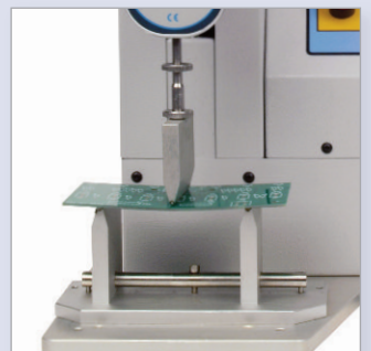
Flexure/bend test of a printed circuit board
