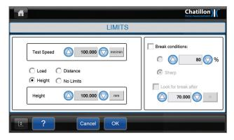
Conduct a quick test by simply entering the type of test, pre-load (if any) and limits.
