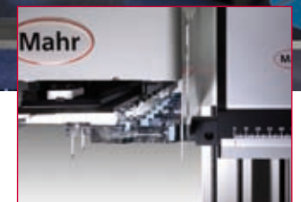
Automatically changing the probe arm enables the CNC measuring run to be performed without interruption.
