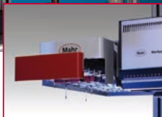
CNC measuring station with MarSurf UD 120 / LD 120 and TWE probe arm changer.
