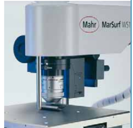
Measuring the honing texture in a bushing that has been split open
