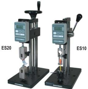
The ES20 is shown in a peel testing application with Series MG digital force gauge, and film & paper grips.
