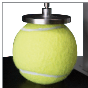
Tennis ball compression test
