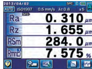
4-parameter display: four parameter measurement results
