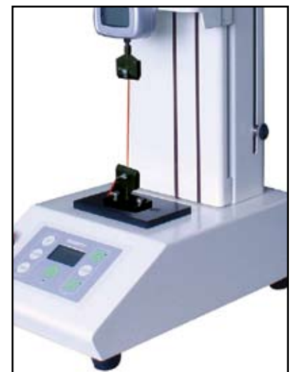
Stand with Optional Grip Performing Tension Test
