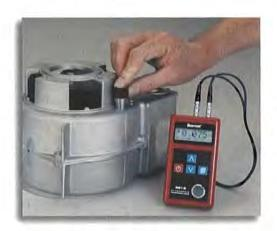
After a simple calibration to a known thickness or sound velocity, the 3812 Ultrasonic Thickness Gage accurately displays readings in either inch or millimeter.
