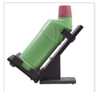
Bleach bottle test fixture
