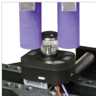
Rotary switch testing
