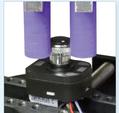
Rotary switch test
