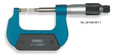
Use Fowler No. 52-246 Blade Micrometers to measure the outside diameter of workpieces which have narrow grooves, "T" slots and other dimensions blocked by shoulders or lands where standard type micrometers cannot be applied.
