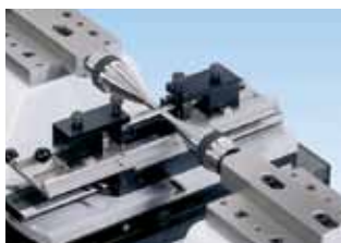
Checking of plug gages and threaded plug gages between centers up to max. dia. 1.18"/30mm, max. length 6"/150mm using 54-197-011, 54-197-806 & 54-197-007
