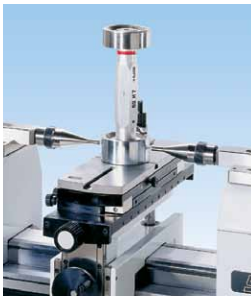
▲ Checking of plug gages and threaded plug gages from dia. 1.18"/30 to 250mm using 54-197-011, 54-197-142, 54-190-806 & 54-197-007
