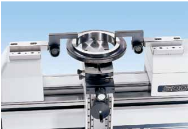
▲ Checking of ring gages from dia. .473"(12mm) to 10"(250mm) using 54-197-011, 54-197-142 & 54-197-162
