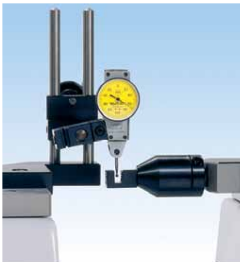
▲ Checking of lever (test) dial indicators using 54-197-115
