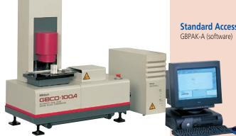
The GBCD-100A Automatic Gage Block Comparator is an easy-to-operate dualhead type gage block inspecting system. It automatically compares workpieces with a standard gage block and determines accuracies of such as central length, maximum length, minimum length, and parallelism through the operation of an optional personal computer.
