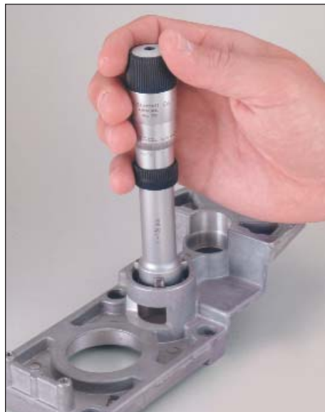
78XTZ-138 Measuring a bore.
