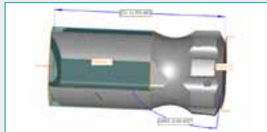
Mining industry drill bit reverse engineered by scanning
