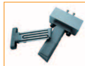
Tool with conformal cooling
