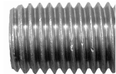
Minor thread nicking on external threads may still be found acceptable.
