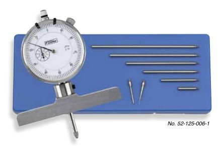
Fowler's X-Depth 22 Dial Depth Gage comes with six interchangeable rods with a 0—22" capacity, carbide contact point and 2 extra points for small applications. Provides rapid measurement of hole depths.
