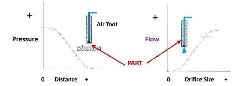
Pressure is created and increases as the distance between the nozzle/orifice and
