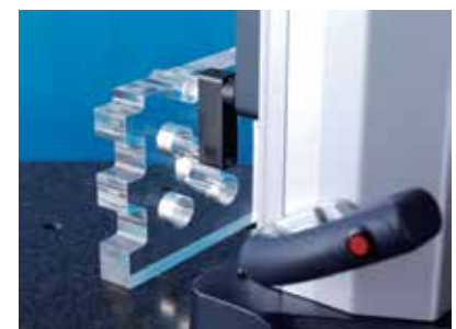
Inside diameter measurement
