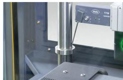
Tactile measurements with T7W
