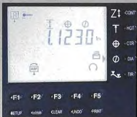
Large, easy-to-view/understand display shows the diameter of a hole or boss.
