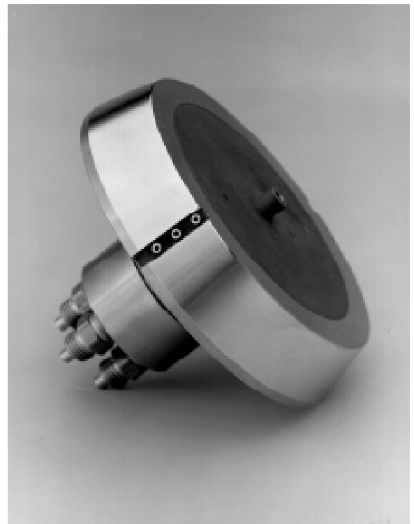
Air plug for measuring a taper
