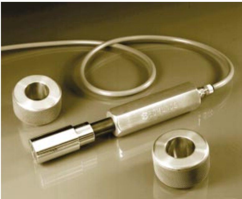
Two-nozzle air plug, with masters, for measuring an inside diameter
