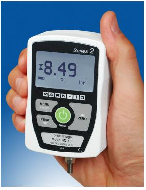
Series 2 digital force gauges are designed for basic tension and compression force testing applications up to 500 lbF (2,500 N). Peak tension and compression readings are reliably captured via the gauges'  $\pm 0.5\%$  accuracy and 500 Hz sampling rate. A backlit graphic LCD displays the current, peak tension, or peak compression reading.
