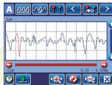
With the Surftest SJ-310, you can delete portions of measurement data. This feature allows you to make new calculations by deleting data that should not be included in parameter calculation, such as data on a scratch.
