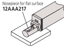
Note 1: Standard accessory for the standard/ retractable drive unit of the SJ-310 Series
