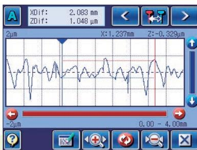
You can not only magnify or shrink waveforms, but also calculate the coordinate difference between two points using a ruler operation. You can quickly check the irregularity status without waiting for a printout.
