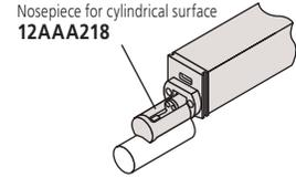
Note 1: Standard accessory for the standard/ retractable drive unit of the SJ-310 Series
