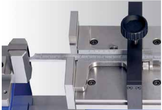
▲ Checking of depth calipers using 54-190-805 & 54-190-827
