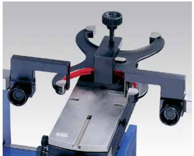
▲ Checking of snap gages from .473 to 6" (12 to 150mm) using No. 54-196-160, 54-190-815 and 54-197-162
