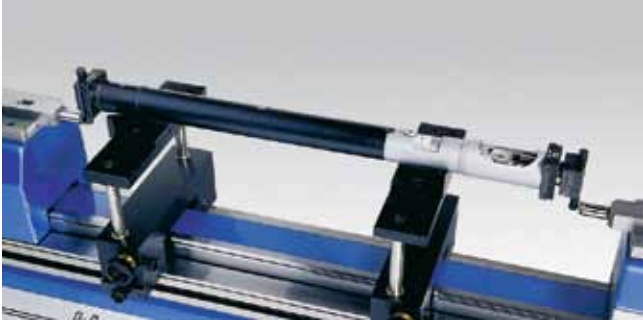
▲ Setting of 2-point bore gages using 54-196-107 and 54-196-021
