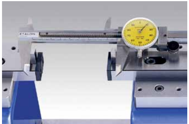
▲ Checking of calipers using 54-196-006
