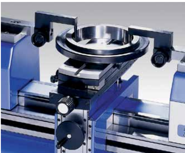
▲ Checking of ring gages from .473 to 10" (12 to 250mm) using No. 54-196-160, 54-197-162 and 54-197-142
