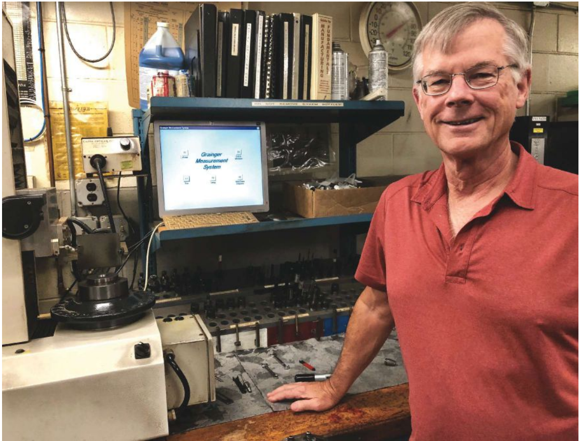
Jake Grainger stands in front of the vision system he created in the early 1990s. Mr. Grainger was one of the first known engineers to develop this type of vision metrology system—a machine that used high-magnification video to aid and assist with the inspection and measurement of small features. The machines feature a camera mounted on a manually operated crankshaft that can be positioned in front of a stage for part inspection. Alpha Grainger still uses several of his original machines today.
