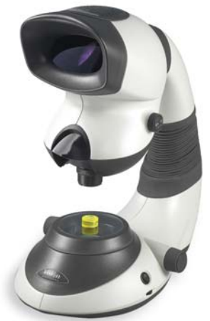
High stability bench stand with integral focus, dimmable substage illumination.
