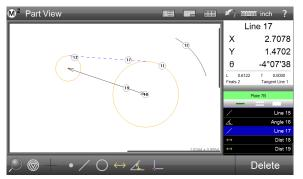
**Graphics-based "Part View" constructions** Generate popular construction types, like Distances and Tangent Lines, from within the graphical part view.
