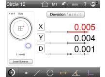
**Geometric tolerancing** Measure features, set nominals, apply tolerances and view deviation results with only a few quick clicks.
