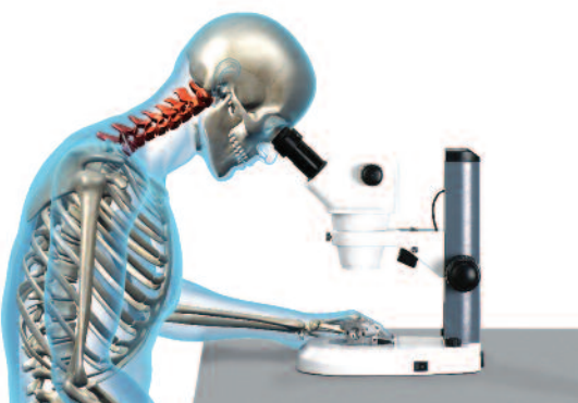
Restrictive eyepieces of a conventional stereo microscope
