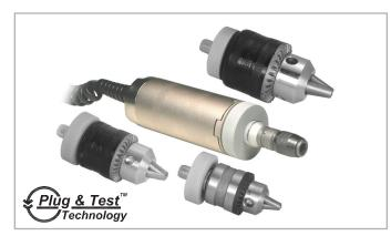
Series R51 smart sensors measure bi-directional torque for numerous applications across virtually all industries. Interchangeable Jacobs chucks and bit holder add flexibility for a variety of applications. The sensors can be used as hand held devices or mounted to a test stand. Superb overload protection adds peace of mind. Capacities available from 10 ozFin to 100 lbFin [7 to 1150 Ncm]. Compatible with Mark-10 indicators (sold separately) through unique Plug & Test<sup>™</sup> technology.
