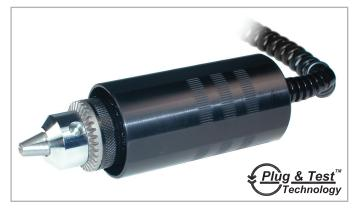
Series R50 smart sensors measure bi-directional torque for a wide variety of applications across virtually all industries. Contain a Jacobs chuck for up to 0.5 in [12.7 mm] diameter samples, bits, or fixtures. The sensors can be used as hand held devices, or mounted to a test stand. Capacities available from 10 ozFin to 100 lbFin [7 to 1150 Ncm]. Compatible with Mark-10 indicators (sold separately) through unique Plug & Test<sup>™</sup> technology.
