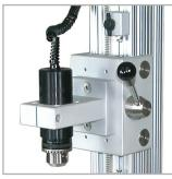
^ A Series R50 torque sensor is shown mounted to a model TSTM motorized torque test stand. The sensor fits into the stand without the need for additional adapters.
