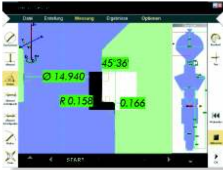
Definition of the measuring areas for measurements of angles, distances and radii
