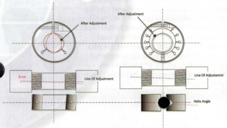
The "Southern style" sets round and stays round through all adjustments due to eccentric design and opposing pressures of the adjusting and locking mechanisms.
