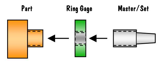
The ring gage inspects the product, and the set plug / master plug / truncated plug inspects the ring gage. Maybe because it is commonly known as the 'set plug', many lab technicians think the set plug is only for the purpose of setting the ring to the proper size. It also has the function of inspecting the ring gage for wear.
