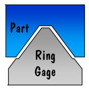
As a ring gage is used it wears, but it can be readjusted to be brought back into size. This means that the wear can continue until the flank is no longer a straight line. This is commonly referred to as the flank having a step wore in it.
