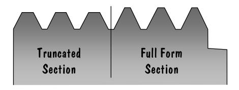
The above picture is a cut-away view of the thread form of the truncated set plug. The thread pitch diameter is the same on both sections and requiring back taper. Back taper is when the measured size of the pitch diameter is less on the back, close to the shank, than on the front. The allowable taper is half of the tolerance of the pitch diameter. Set plugs with front taper should be replaced.
