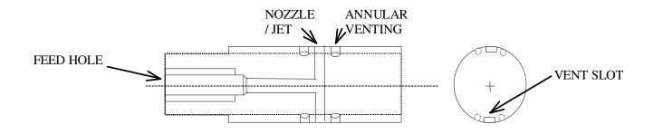
An Air Tool holds these nozzles in a precise steel cylinder or ring.
