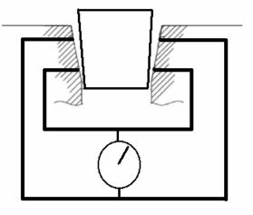
Lower set of jets see more back pressure than the upper set of jets. Meter on Dimensionair indicates smaller taper angle
