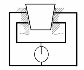
Upper set of air jets and lower set of air jets in air ring see the same back pressure. Meter on Dimensionair reads zero
