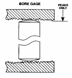
An air gage averages a measuring area A mechanical contact gage is a point contact system and measures the high points
