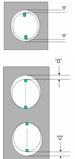
Because two jets are used to measure diameter – another form of differential check – the condition shown will display the same reading in each case.
