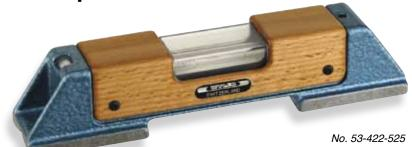
The Fowler-Wyler Horizontal Spirit Level is used for inspecting and levelling horizontal surfaces and cylinders. Sensitivity of .0005" per 10" length. This model features prismatic bearing surface, longitudinal and cross levels. Levels feature numerous advantages and ensure easy, accurate measurements.
