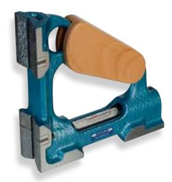
WYLER Magnetic Precision Spirit Level checks and levels cylinders, horizontal and vertical surfaces. Constructed with two prismatic measuring surfaces. Sensitivity .0002" per 10". Magnets to ensure complete adherence to vertical surfaces of parts and vertical arbors or shafts. Operators on milling and boring units, inspectors and fitters work with free hands.
