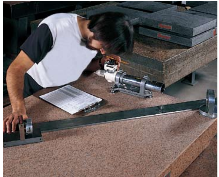
Inspecting a granite plate with an autocollimator
