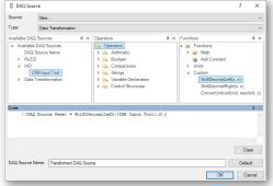
Transform data from measurement sources before storing and displaying results. This function can convert units and shift decimal points to make data collection even easier.
