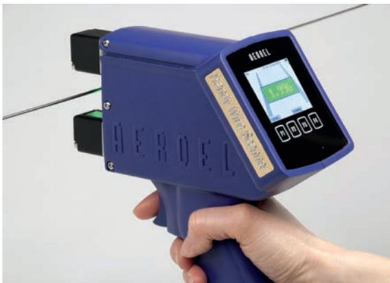
**HWS.1 - Handy Wire Scanner** is a fully portable optical micrometer for non-contact measurement of wires, cables and other similar products.
