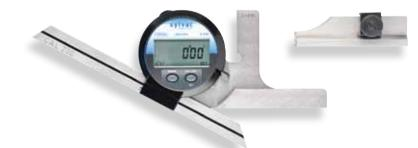
Fowler-Sylvac's Deluxe Electronic Protractor, featuring the patented Sylvac measuring system, provides an LCD readout in 1 minute of arc or 0.01 degrees of arc. A push-button selects the range according to application  $(1 \times 360^\circ, 2 \times 180^\circ \text{ or } 4 \times 90^\circ)$  and changes the reading from arc minutes to decimal degrees. Additional push-buttons provide "reset" and "print" functions.
