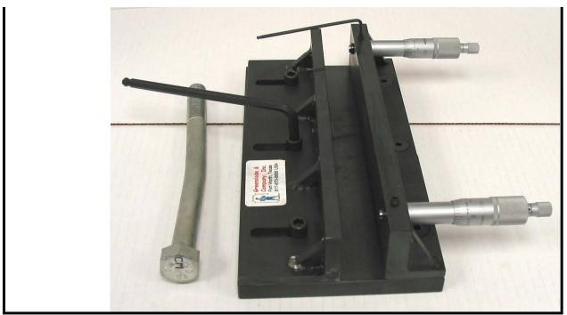
This gage is used to inspect for the straightness or camber in a bolt or screw. The allowance for bend or camber is specified in the various product standards.
