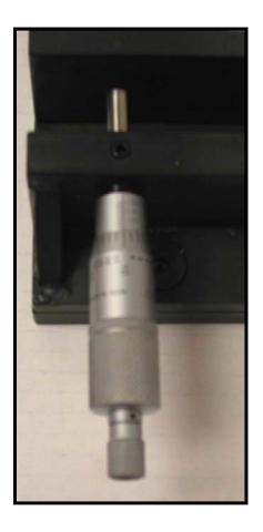
4. Press the movable side firmly against the ends of the micrometer heads and tighten the three lock down screws to affix the moveable side into place.
