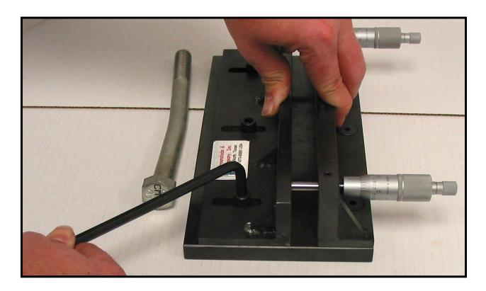
5. To inspect the part slide it in from either end of the gage to the position where two diameter lengths of the part remain outside the gage. If the part will rotate a full 360 degrees the part is acceptable for straightness or camber.
