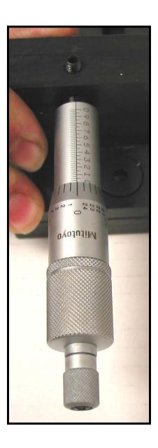
2. Firmly press the moveable side against the stationary side of the gage. Tighten the set screws to hold the micrometer heads in proper position. The thimble should rotate freely. If it feels tight loosen the set screw slightly.
