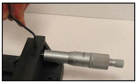
3. To inspect a part slide the moveable side away from the stationary side and set both micrometer heads to the allowable camber for the part which is being inspected.
