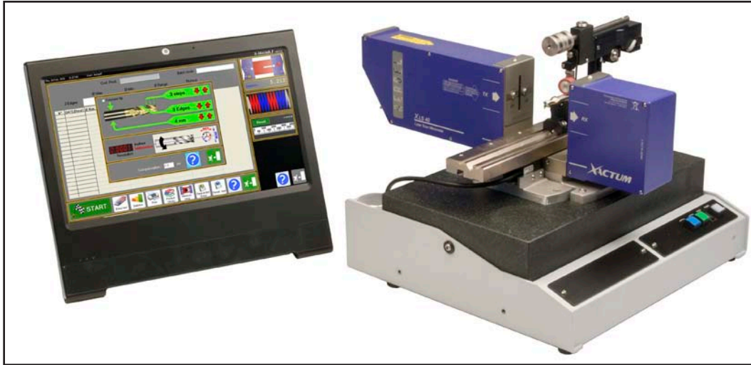
Pictured above is the Aeroel Super Meclab T40. It shows the XLS 40 laser gauge head with a granite based precision linear slide, cutting tool fixture and the 15" touch screen display unit.
