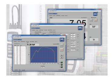
The programs include a set of tools to analyze test results, including statistical calculations, quick data export to Microsoft Excel, customizable reports, pass/fail indicators, and many others. Test setups are customizable and can be saved and recalled. The user can program test start and stop conditions, including load, time, distance, and sample break. Additional features include a large display screen for real time load and travel data and a utility to configure Mark-10 gauges from a PC.
