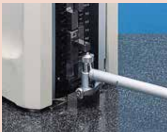
Bore gage zero-setting
