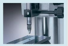
Difference measurements with opposite polarity signs (+A -B)
