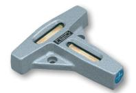
Model C:T-shaped level with cross vials, 2-point mounting. Manually lapped measuring base to ensure a much higher precision of the level.
