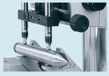
Establishing form and position errors with "max - min" memory function as in the example for runout errors
