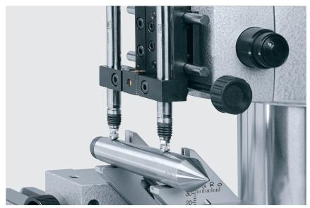
Measurement of difference between two inductive probes
