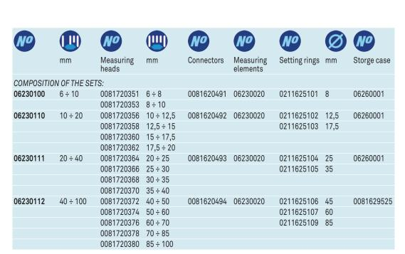
Set available on request for extending the application range from 100 to 300 mm.
