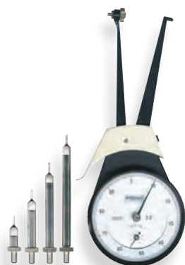
▲ No. 52-552-001 supplied with five interchangeable anvils.
