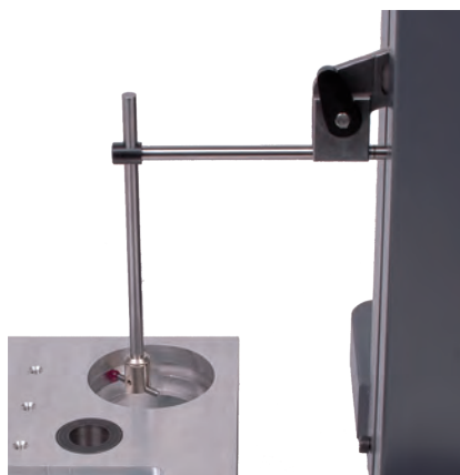
Internal groove measurements with accessories 54-199-508, 54-199-506 and 54-199-501
