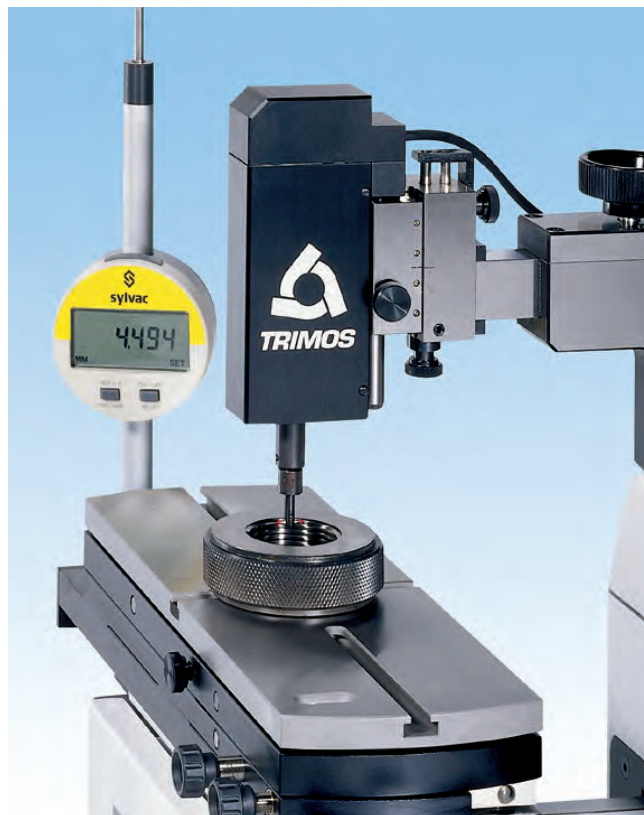
▲ Checking of threaded ring gages from pitch 0.7 to 6mm/48 to 4 threads per inch (max. internal dia. 7.08"/180mm) using table (54-197-011), clamps (54-197-142), Internal measuring device (54-197-074) & T-Ball probes (54-197-075)
