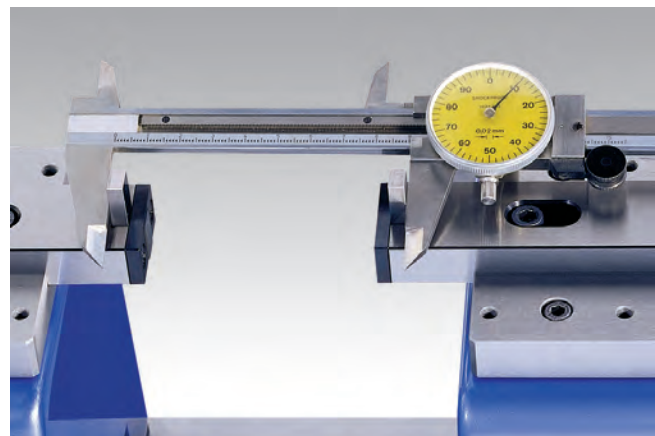
▲ Checking of calipers using 54-196-006
