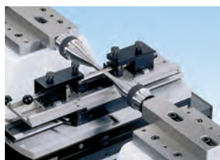
Checking of plug gages and threaded plug gages between centers up to max. dia. 1.18"/30mm, max. length 6"/150mm using table (54-197-011), small Ø anvils (54-197-806) & thread wires (54-197-007)
