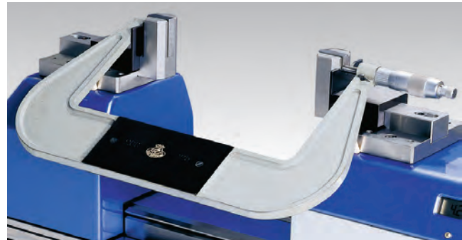
▲ Checking and setting of external micrometers from 3" to 120"(75 to 3050mm) using gage block anvils (54-190-805) & micrometer V-supports (54-190-825)
