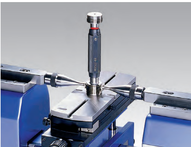
▲ Setting of threaded plug gages from diameter 1.18" to 9.84" (30 to 250mm) using table (54-196-160), small Ø anvils (54-190-806) and thread wires (54-197-007)
