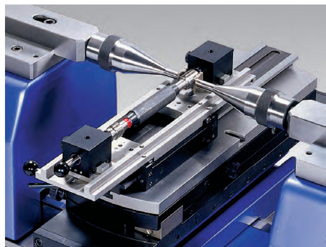
▲ Setting of threaded plug gages between centers up to maximum diameter of 1" (26mm), maximum length 6" (150mm) using table (54-196-160), small Ø anvils (54-190-806), thread wires (54-197-007) and plug holder (54-197-006)
