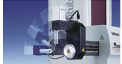
Holder-arm orientation switching (vertical position - horizontal position)
