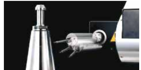
Detector rotation mechanism (0 to 290°, in increments of 1°)
