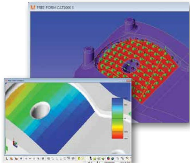
Surface deviation can be displayed as spherical points or as a gradient surface.
