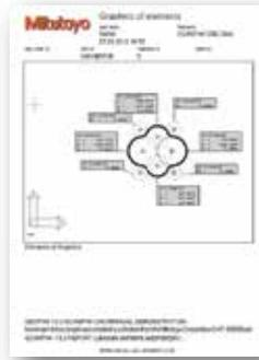
SCANPAK constructs from the measured contour circles and/or line elements based on the user-specified tolerance amount calculated from the elements form deviation.
