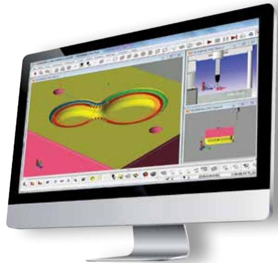
The contour compared to the nominal "AS IS." The areas shown in red fail to meet the profile requirement.
